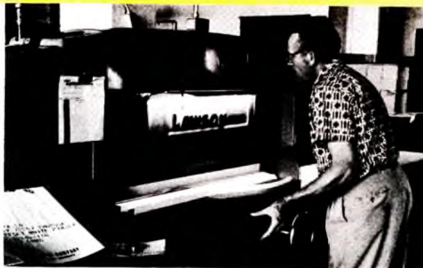
Power-driven paper cutter trims periodicals or cuts stock to page size before press run.
