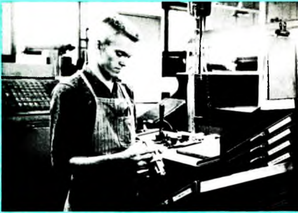
Ludlow operator assembles a line of headline type
