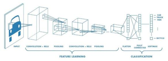
Figure 6: Visualization of layers of a CNN (Prabhu)
